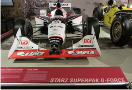
This 2001 Starz Superpak G-Force was one of the first designs to simulate an inverted airplane wing, which causes downward force on the car. It has revolutionized racing.
