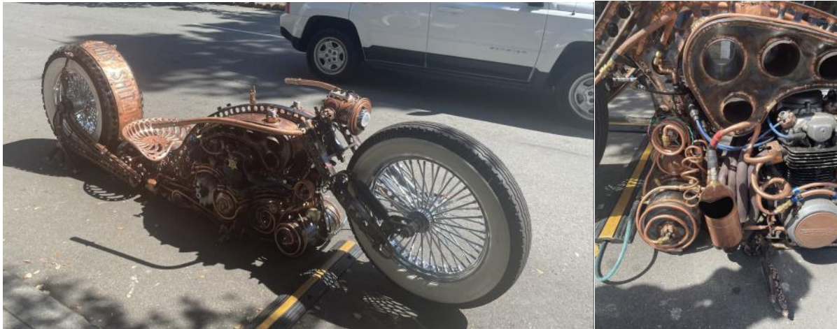
The things people cook up in their spare time. Street legal (sort of), tractor seat, air suspension, flame thrower exhaust, etc...
